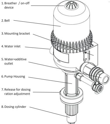
You are now the owner of a Mixtron Volumetric Dosing Pump.
