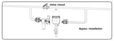
To ensure the dosing pump's proper operation and maximum life, it is advisable to install a filter (we recommend 60-130 microns) on the delivery line and upstream of the dosing pump. Observe the standards and regulations in force in your country when connecting to the public water supply network.
