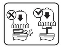
When re-assembling the top bell (G) you can use a strap wrench to help applying the
