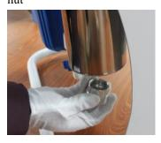
Step 8: Screw the nuts tightly on the reactor chamber. Firm hard tightness is sufficient. Tools should not used so as to avoid damaging the quartz sleeve
