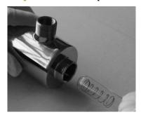
**Step 7:** Hand-screw the end nut onto the Reactor Chamber. In order to protect the O-ring, do not over tighten.
