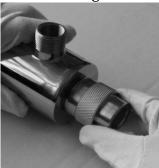
**Step 8:** Connect the 4-pin electrical socket with the UV lamp pins tightly.
