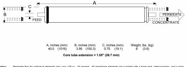
Notice: Permeate flow for individual elements may vary +25 or - 15 percent. All membrane elements are supplied with a brine seal, interconnector, and o-rings. Elements are enclosed in a sealed polyethylene bag containing less than 1.0% sodium meta-bisulfite solution, and then packaged in a cardboard box. All elements are guaranteed 99.4% minimum rejection.
