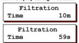
The second line indicates the remaining time for the phase "Filtration" will start. When the start is within 60 seconds the remaining time will be displayed in seconds.
