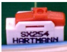
Switch position right (delivery status)
