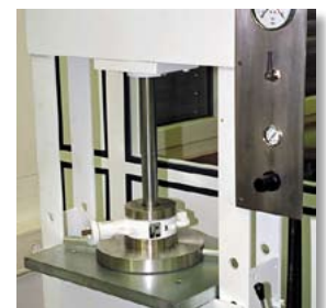
Tightness test with HP nitrogen
